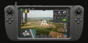
The C-NAVIGATOR is a ground control station intended for industrial use, optimizing the user with its sleek and improved ergonomic design. Offering 2x 2-Axis joysticks, 2x 1-Axis joysticks and 12x buttons, the C-NAVIGATOR is made to meet customers' need for mapping out the buttons.
